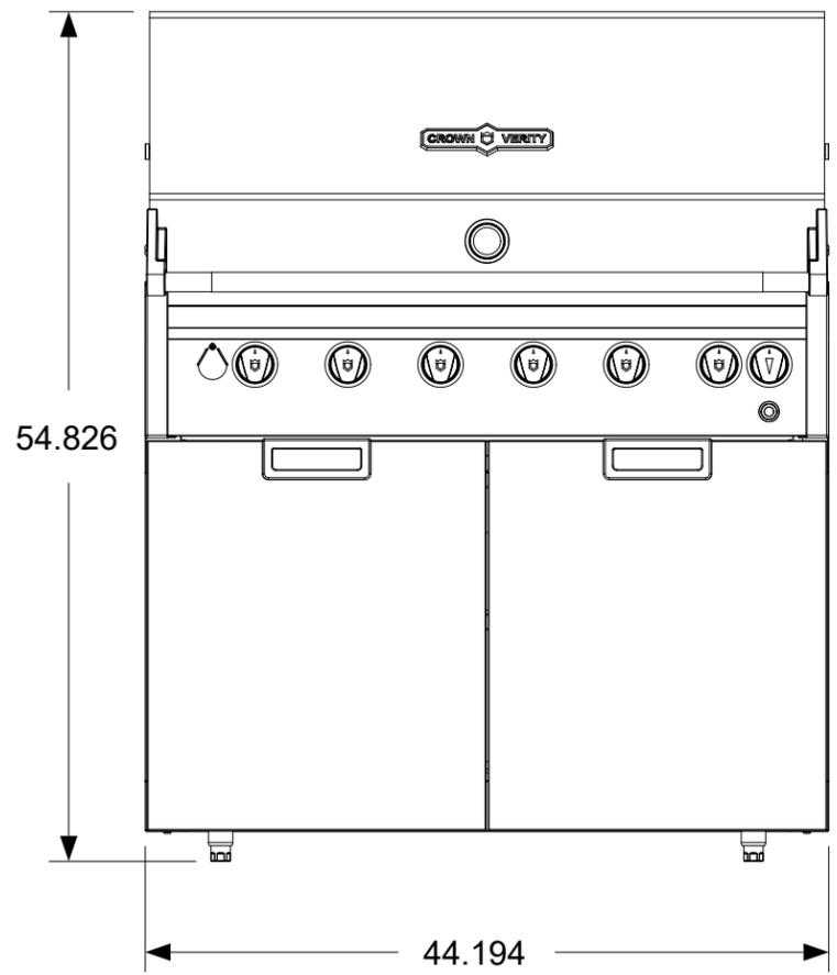
Adjustable leveling leg shown at lowest setting. Adjustment range is 2.125 inches.
