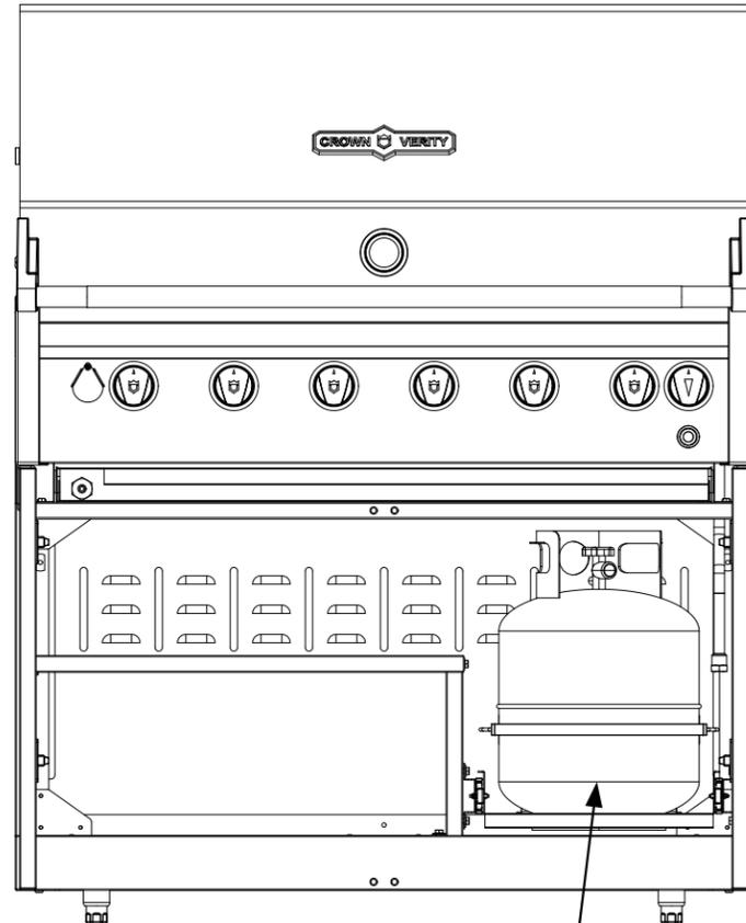
For LP applications that are not connected to a bulk supply, a pull-out propane tank drawer is factory installed along with a hose and regulator assembly to attach to a 20 lbs. tank (not supplied). A shelf is also installed to prevent the storage of a second propane tank per the residential standard for outdoor cooking appliances ANSI Z21.58-2018 and CSA 1.6-2018
