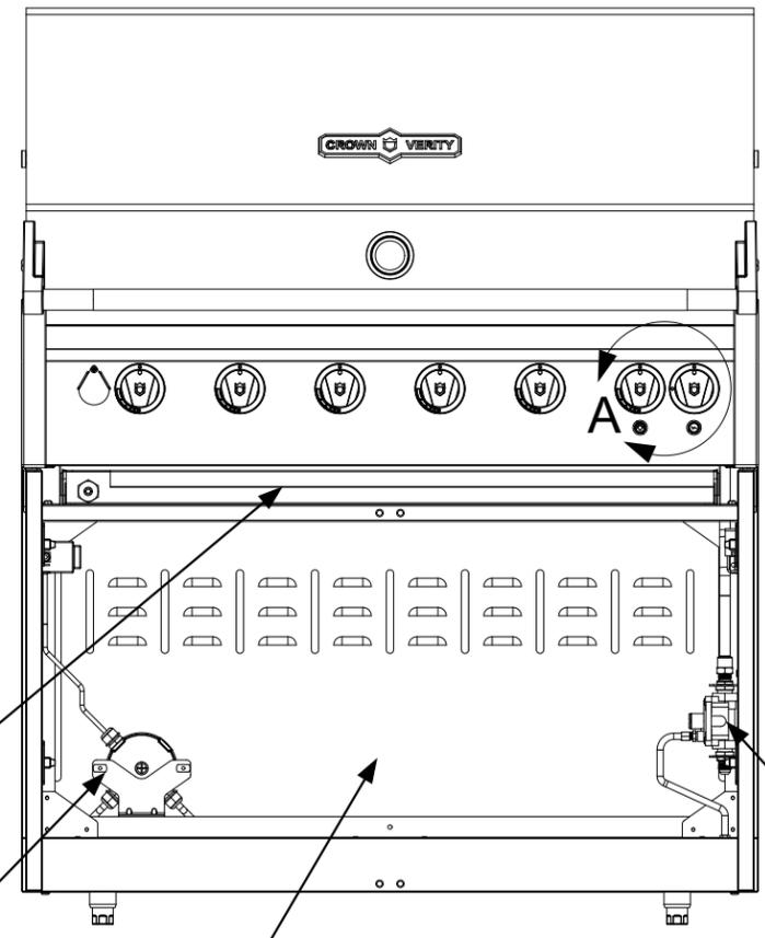
Natural gas connection shown. For propane versions, bulk tank connections would also occur here. For propane versions not connected to a bulk tank, a pull-out propane tank drawer is provided along with a hose and regulator assembly to attach to a 20 lbs. tank (not supplied).
