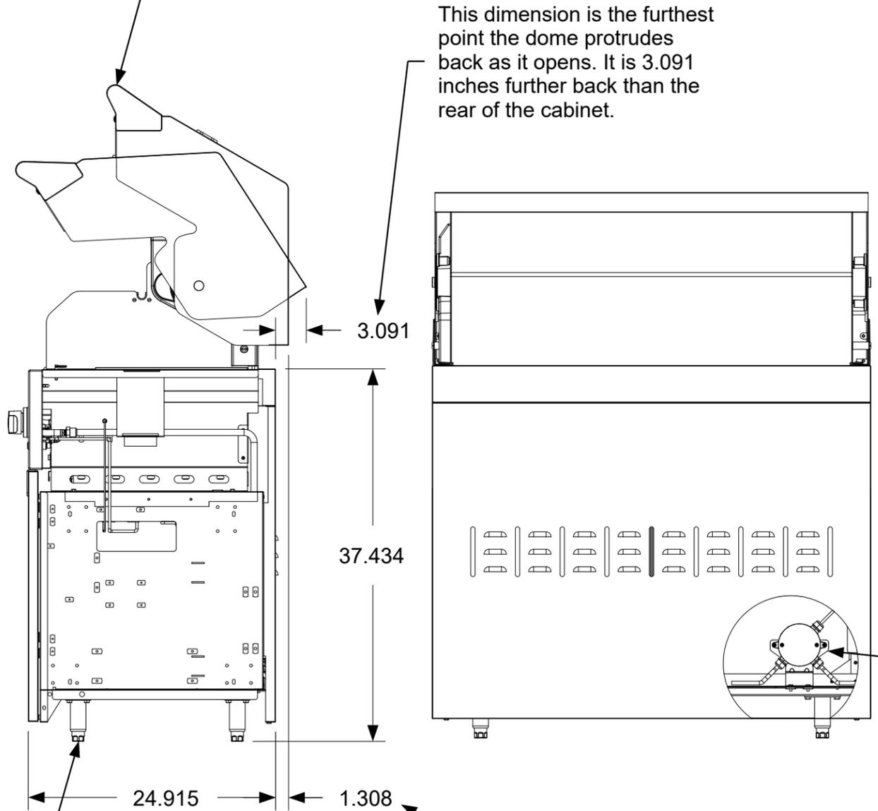
This dimension is the furthest point the dome protrudes back as it opens. It is 3.091 inches further back than the rear of the cabinet.
