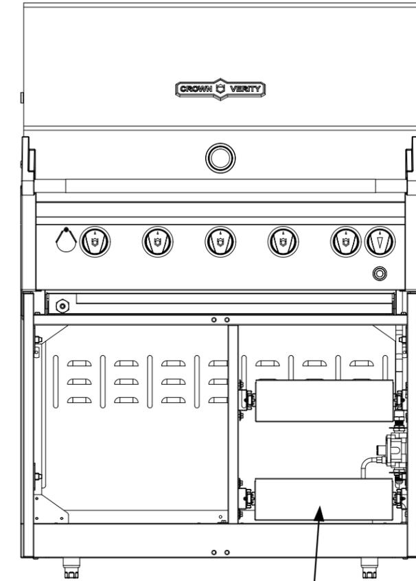
Storage area below the grill is shown with the optional utility drawer. The cabinet can accommodate a single or dual drawer as shown.
