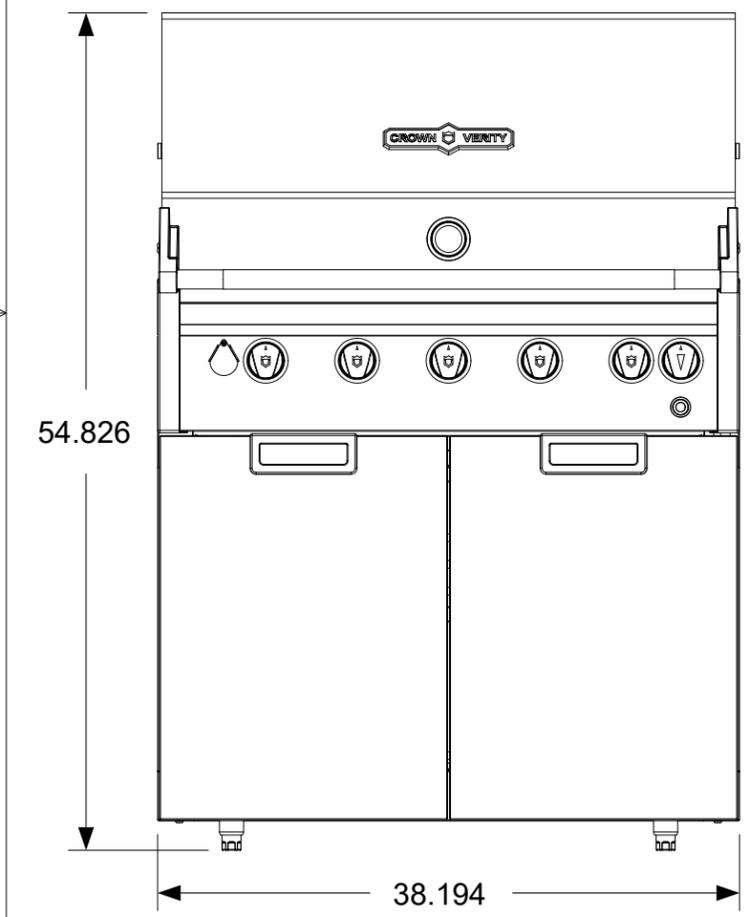
Adjustable leveling leg shown at lowest setting. Adjustment range is 2.125 inches.
