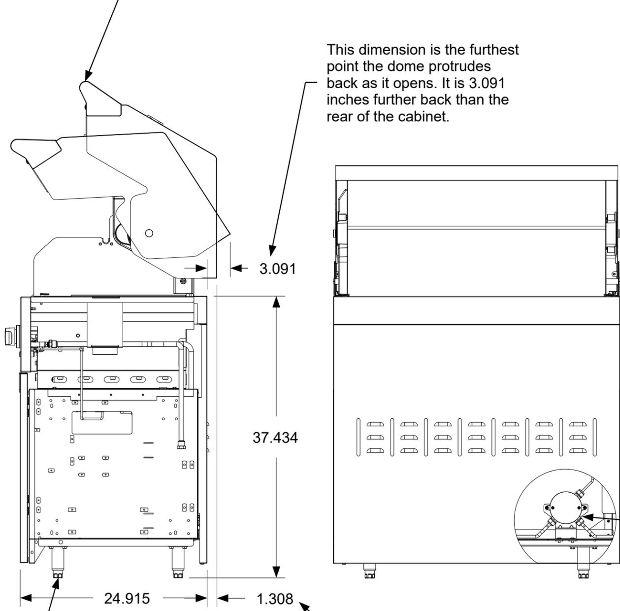
This dimension is the furthest point the dome protrudes back as it opens. It is 3.091 inches further back than the rear of the cabinet.
