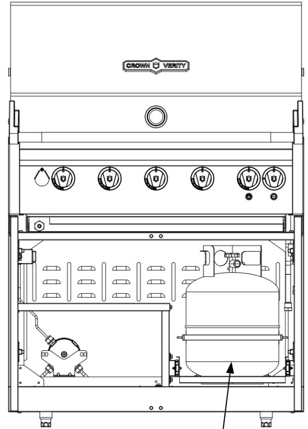
For LP applications that are not connected to a bulk supply, a pull-out propane tank drawer is factory installed along with a hose and regulator assembly to attach to a 20 lbs. tank (not supplied). A shelf is also installed to prevent the storage of a second propane tank per the residential standard for outdoor cooking appliances ANSI Z21.58-2018 and CSA 1.6-2018
