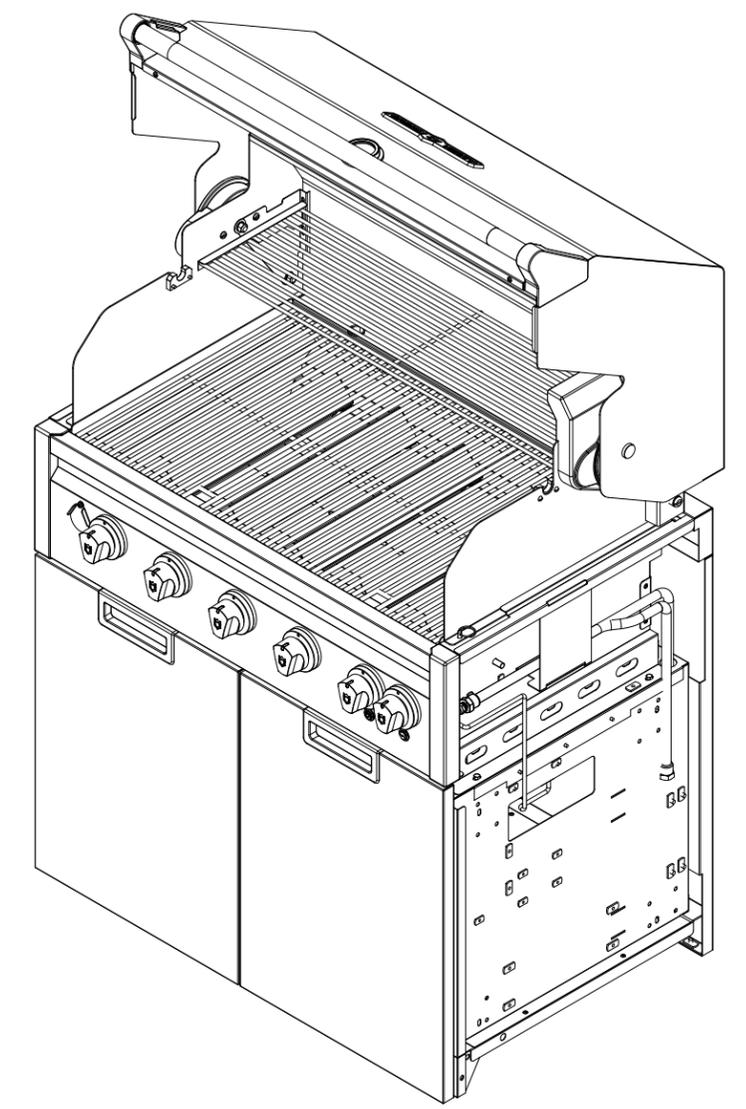
The junction box for electrical connections is located behind the removable back panel. A section of the back panel has been removed for clarity.
