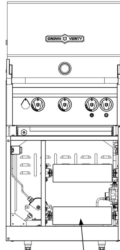
For LP applications that are not connected to a bulk supply, a pull-out propane tank drawer is factory installed along with a hose and regulator assembly to attach to a 20 lbs. tank (not supplied).
