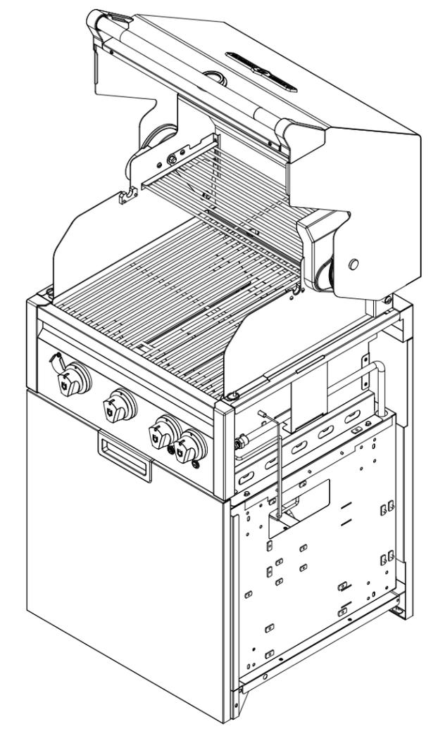
The junction box for electrical connections is located behind the removable back panel. A section of the back panel has been removed for clarity.
