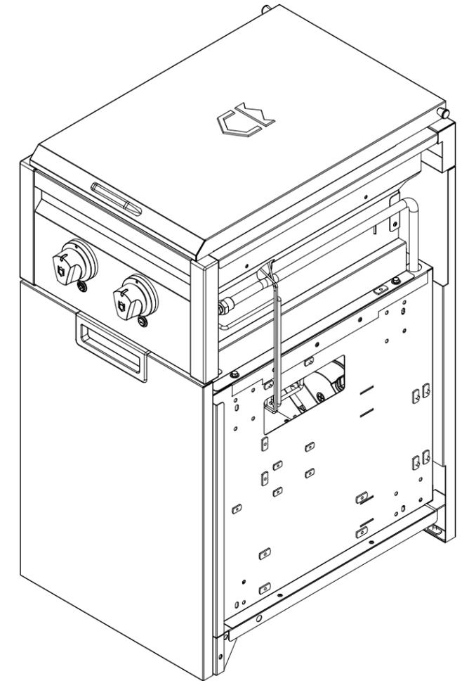
The junction box for electrical connections is located behind the removable back panel. A section of the back panel has been removed for clarity.
