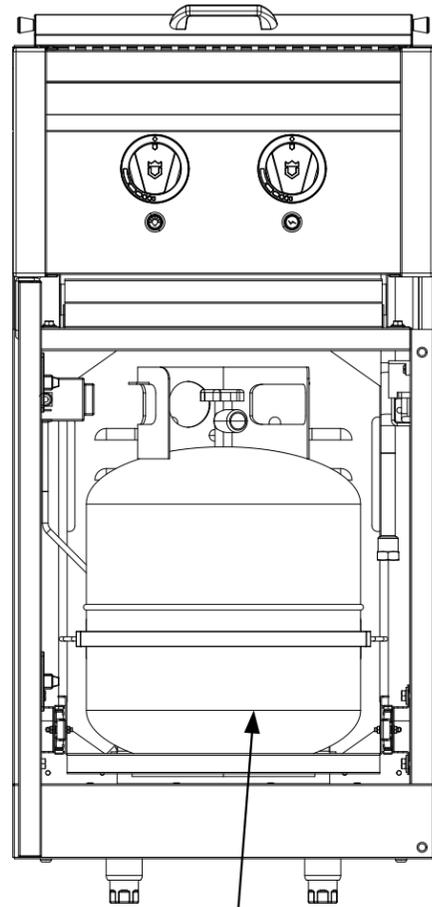
For LP applications that are not connected to a bulk supply, a pull-out tank drawer is factory installed along with a hose and regulator assembly to attach to a 20 lbs. tank (not supplied)
