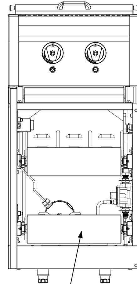
Storage area below the side burner is shown with the optional utility drawer. The cabinet can accommodate a single or dual drawer as shown.
