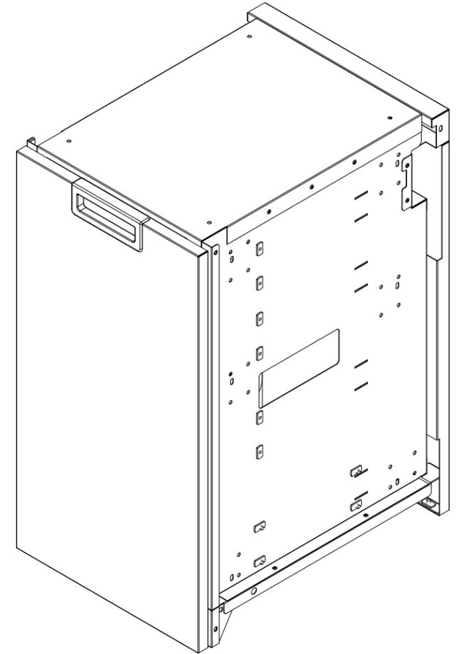
Adjustable leveling leg shown at lowest setting. Adjustment range is 2.125 inches.
