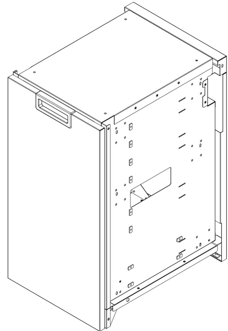
Door shown with righthand mounting option. Door hardware can be switched for lefthand mount.
