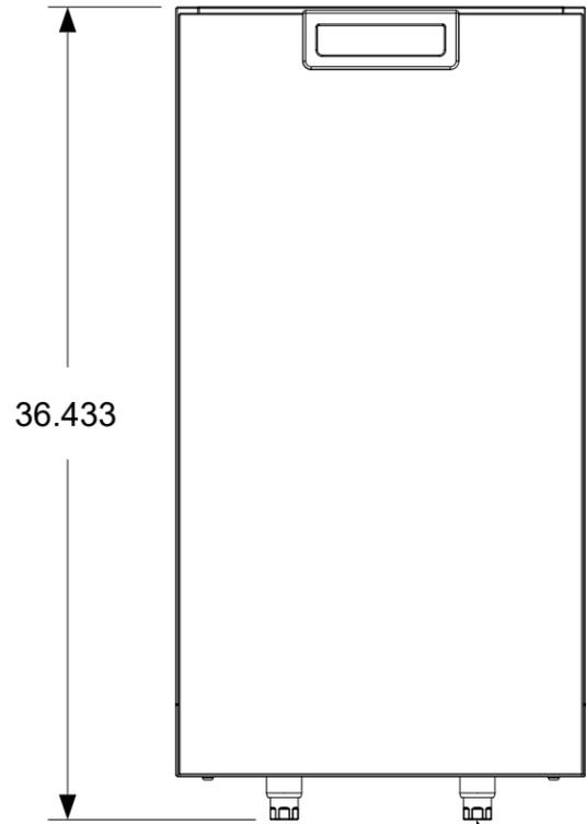
The top of the cabinet has been recessed one inch below the grill, side burner and sink modules to accommodate a one inch thick countertop material to be supplied by the customer.
