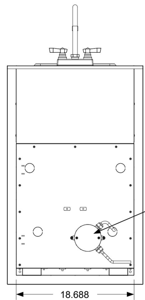
Junction box for electrical connections. Supplied with all hot water tank options and for the non pressurized cold water versions to power the water pump.
