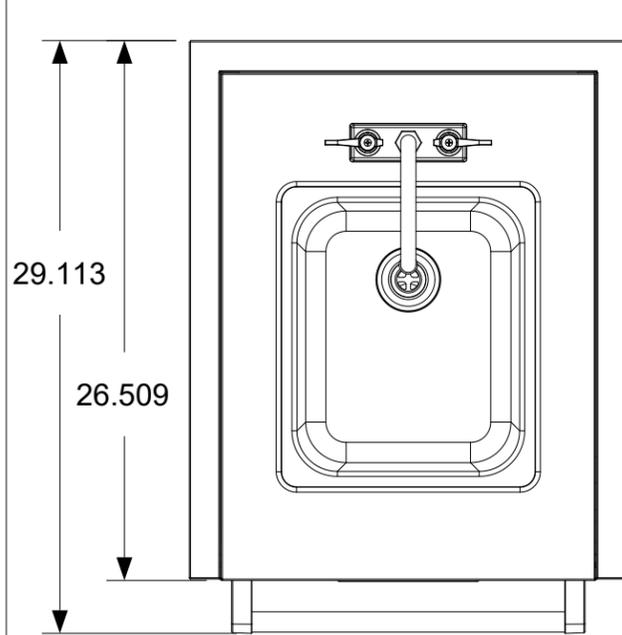
Dimensions shown are the actual physical dimensions. Additional clearances to the cabinetry are dependent on the tolerances of the cut-out. The suggested cut-out dimensions are listed in the chart below but these dimensions can be reduced if the tolerances are controlled. Please refer to the product manual for installation instructions.
