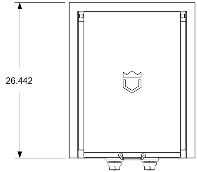
Dimensions shown are actual physical dimensions. Additional clearances to the cabinetry are dependent on the tolerances of the cut-out. The suggested cut-out dimensions are listed in the chart below but these dimensions can be reduced if the tolerances are controlled. Please refer to the installation manual for additional clearances to combustibles and installation instructions.
