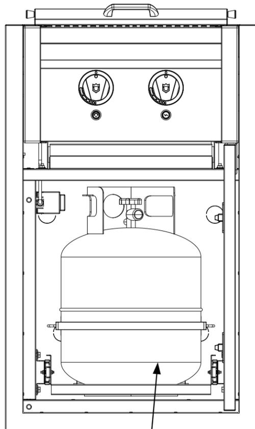
For LP applications that are not connected to a bulk supply, a pull-out tank drawer is factory installed along with a hose and regulator assembly to attach to a 20 lbs. tank (not supplied)
