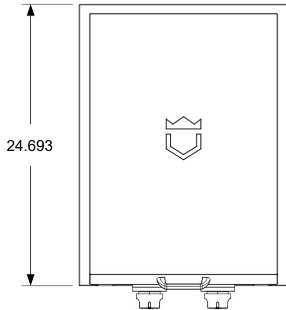
Dimensions shown are actual physical dimensions. Additional clearances to the cabinetry are dependent on the tolerances of the cut-out. The suggested cut-out dimensions are listed in the chart below but these dimensions can be reduced if the tolerances are controlled. Please refer to the installation manual for additional clearances to combustibles and installation instructions.
