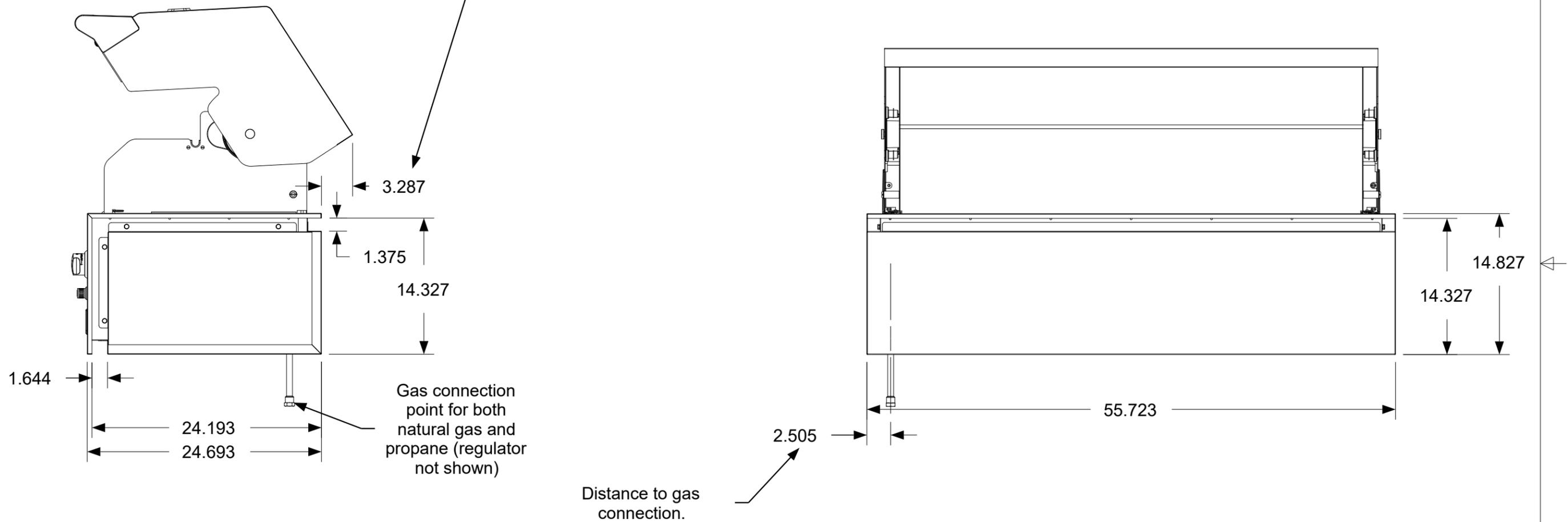
The dimensions shown are the actual physical dimensions of the grill. Additional clearances to cabinetry are dependent on the tolerances of the cut-out. The suggested cut-out dimensions are listed in the chart below but these dimensions can be reduced if the tolerances are controlled.
