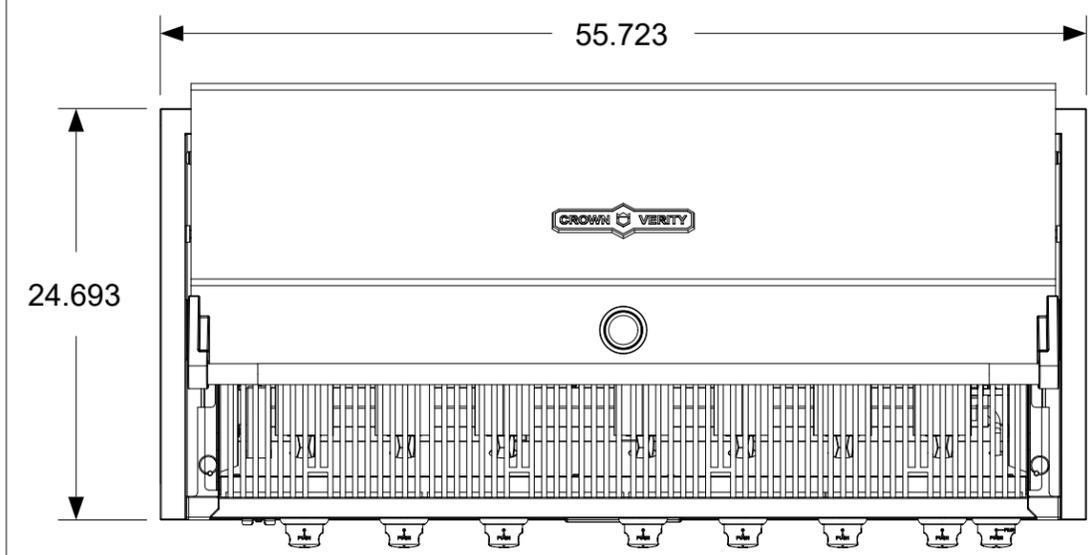
The dimensions shown are the actual physical dimensions of the grill. Additional clearances to cabinetry are dependent on the tolerances of the cut-out. The suggested cut-out dimensions for the insulated jacket option are listed in the chart below but these dimensions can be reduced if the tolerances are controlled.
