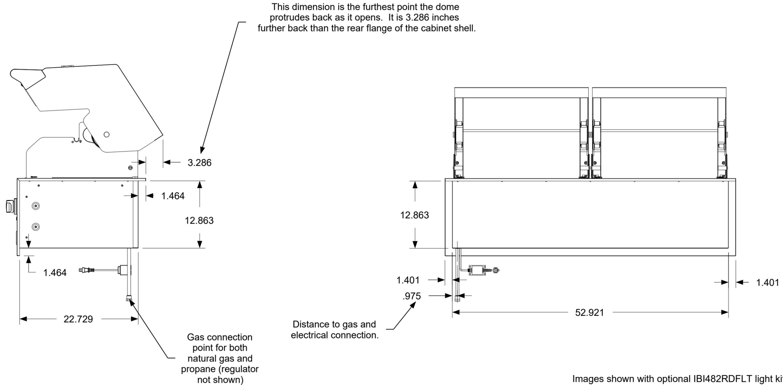
The dimensions shown are the actual physical dimensions of the grill. Additional clearances to cabinetry are dependent on the tolerances of the cut-out. The suggested cut-out dimensions are listed in the chart below but these dimensions can be reduced if the tolerances are controlled.
