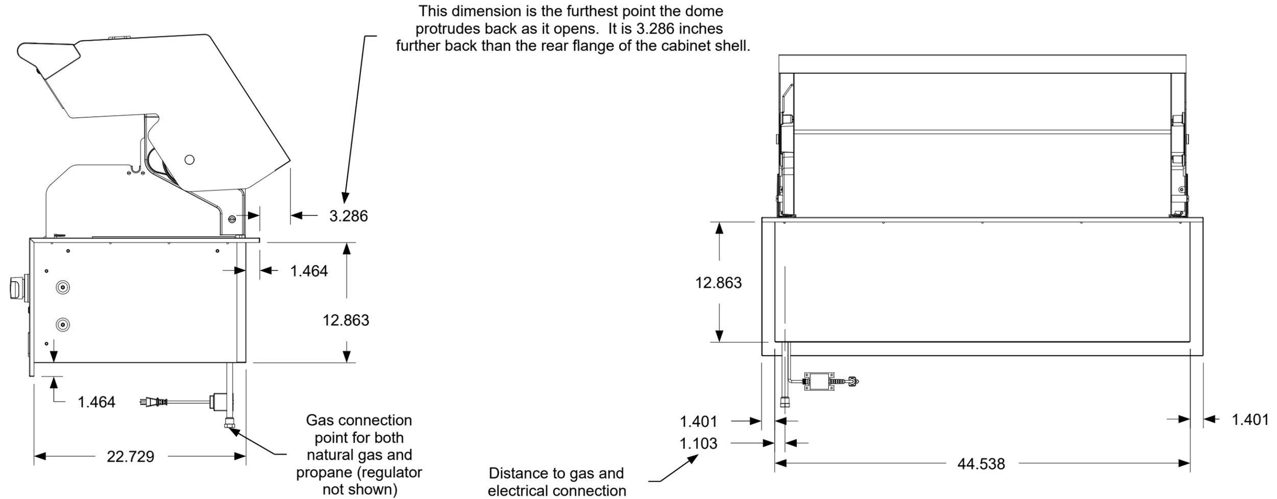
The dimensions shown are the actual physical dimensions of the grill. Additional clearances to cabinetry are dependent on the tolerances of the cut-out. The suggested cut-out dimensions are listed in the chart below but these dimensions can be reduced if the tolerances are controlled.
