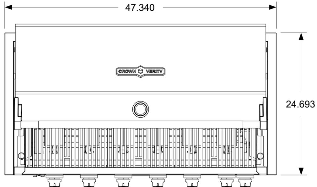
The dimensions shown are the actual physical dimensions of the grill. Additional clearances to cabinetry are dependent on the tolerances of the cut-out. The suggested cut-out dimensions for the insulated jacket option are listed in the chart below but these dimensions can be reduced if the tolerances are controlled.
