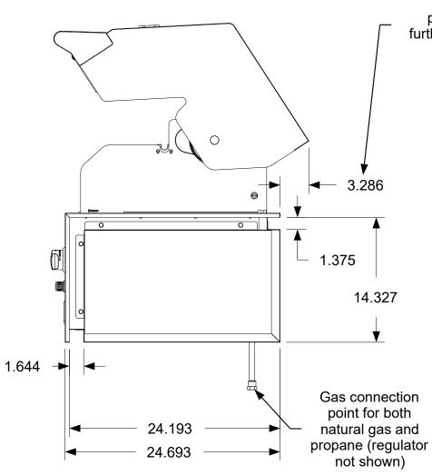
This dimension is the furthest point the dome protrudes back as it opens. It is 3.286 inches further back than the rear flange of the cabinet shell.
