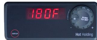
Standard solid state electronic control with large, clear, easy-to-read and operate LED digital display to ensure holding at precise food temperature
