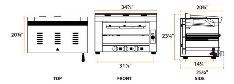
Cooking Performance Group S-36-SB-N 36" Natural Gas Infrared Salamander Broiler with 36" Heat Shield and Mounting Brackets - 36,000 BTU
