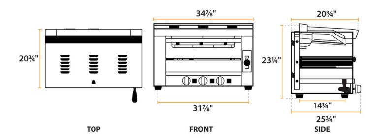
Cooking Performance Group S-36-SB-L 36" Liquid Propane Infrared Salamander Broiler with 60" Heat Shield and Mounting Brackets - 36,000 BTU
