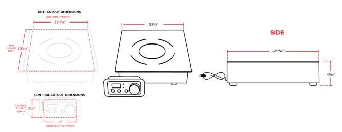
Cooking Performance Group IDCPG-19A Drop-In Induction Range with Remote Control -120V, 1900W
