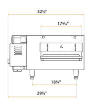
**Cooking Performance Group ICOE-50-D Countertop Impinger Electric Conveyor Oven** with 50" Belt - 240V, 1 Phase, 6700W
