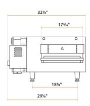
Cooking Performance Group ICOE-50-B Countertop Impinger Electric Conveyor Oven with 50" Belt - 208V, 1 Phase, 6700W
