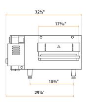
Cooking Performance Group ICOE-32-D Countertop Impinger Electric Conveyor Oven with 32" Belt - 240V, 1 Phase, 6700W
