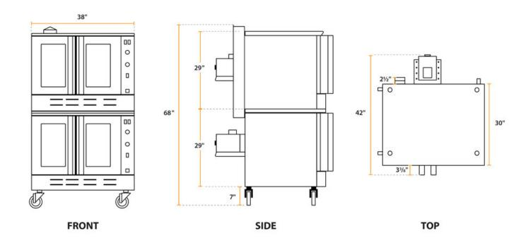
Cooking Performance Group FGC-200-LK Double Deck Standard Depth Full Size Liquid Propane Convection Oven with Legs - 108,000 BTU
