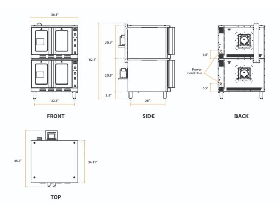
Cooking Performance Group FEC-200-DDDK Deep Depth Double Deck Full Size Electric Convection Oven - 240V, 1 / 3 Phase, 20.2-23.8 kW
