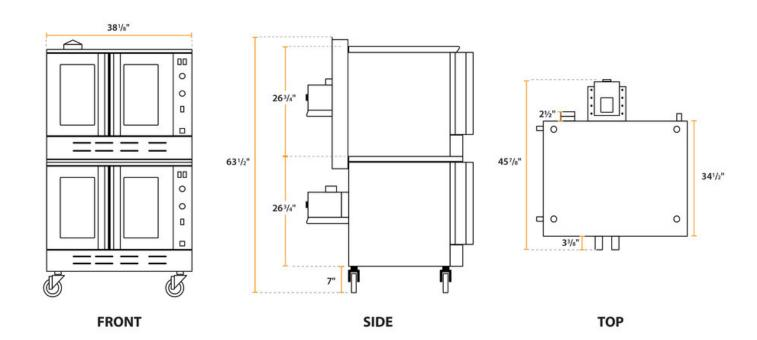
Cooking Performance Group FEC-100-DDCK Deep Depth Double Deck Full Size Electric Convection Oven - 208V, 3 / 1 Phase, 11 kW
