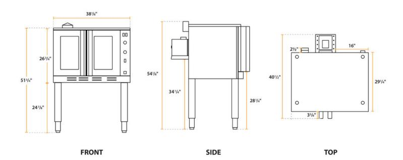
Cooking Performance Group FEC-100-E Single Deck Standard Depth Full Size Electric Convection Oven -240V, 3 Phase, 11.9 kW
