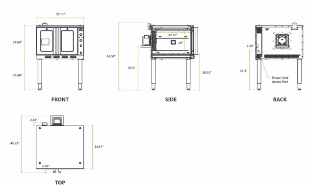
Cooking Performance Group FEC-100-DDD Deep Depth Single Deck Full Size Electric Convection Oven - 240V, 1 / 3 Phase, 10.1-11.9 kW
