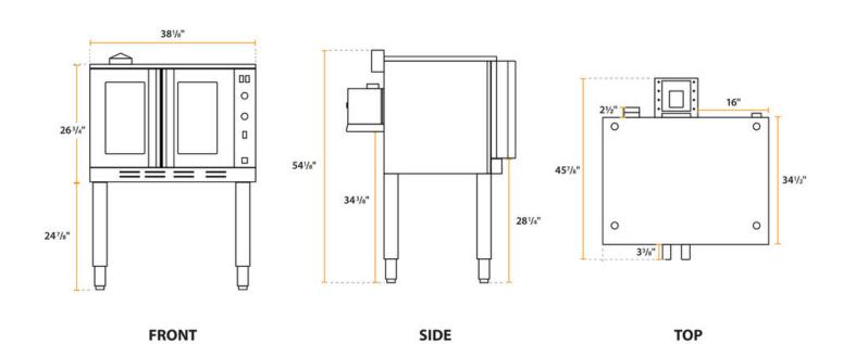
Cooking Performance Group FEC-100-DDC Deep Depth Single Deck Full Size Electric Convection Oven - 208V, 3 / 1 Phase, 11 kW
