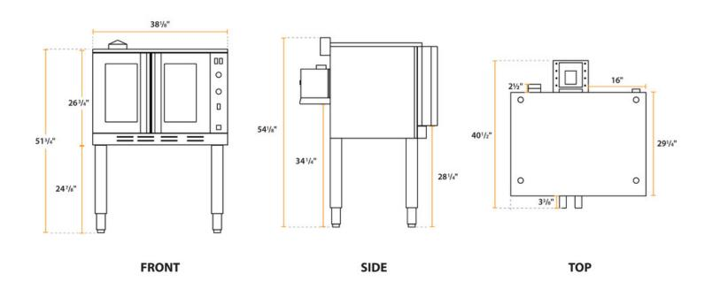
Cooking Performance Group FEC-100-B Single Deck Standard Depth Full Size Electric Convection Oven -208V, 1 Phase, 11 kW
