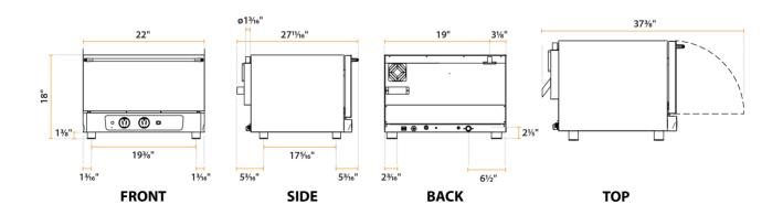
Cooking Performance Group COH-D3-A Electric Digital Countertop 3 Tray Half Size Convection Oven with Steam Injection - 120V, 1650W
