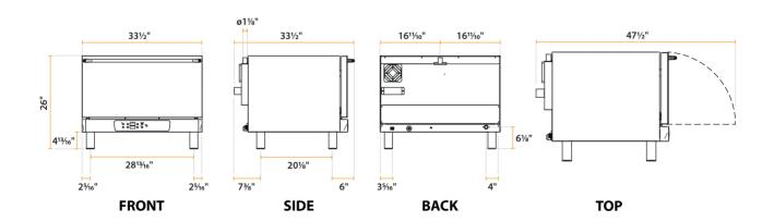
Cooking Performance Group COF-T4-M Electric Thermostatic Countertop 4 Tray Full Size Convection Oven with Steam Injection - 208-240V, 5600W
