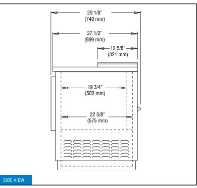
**IMPORTANT:** Model is completely front breathing and intakes and exhausts air through the front grill. A clearance of 1" on the back and 3" on the sides is recommended.
