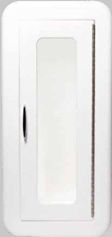
SPECIFICATIONS: Fire Extinguisher Cabinet, as manufactured by Cato, Inc., with body, bezel and door, injection molded of white virgin 2 Izod Co-Polymer Polypropylene of .15 wall thickness, virgin acrylic Plaskolite panel of .080 thickness, stainless steel hinge, chromium-plated door handle and roller catch.
