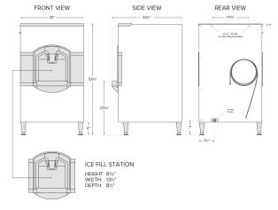
INSTALLATION NOTE: ALLOW 6" SPACE AT LEFT, BACK, AND RIGHT SIDES FOR VENTILATION AND UTILITY CONNECTION
