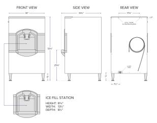
NSTALLATION NOTE: ALLOW 6" SPACE AT LEFT, BACK, AND RIGHT SIDES FOR VENTILATION AND UTILITY CONNECTION
