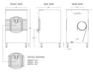
INSTALLATION NOTE: ALLOW 6" SPACE AT LEFT, BACK, AND RIGHT SIDES FOR VENTILATION AND UTILITY CONNECTION
