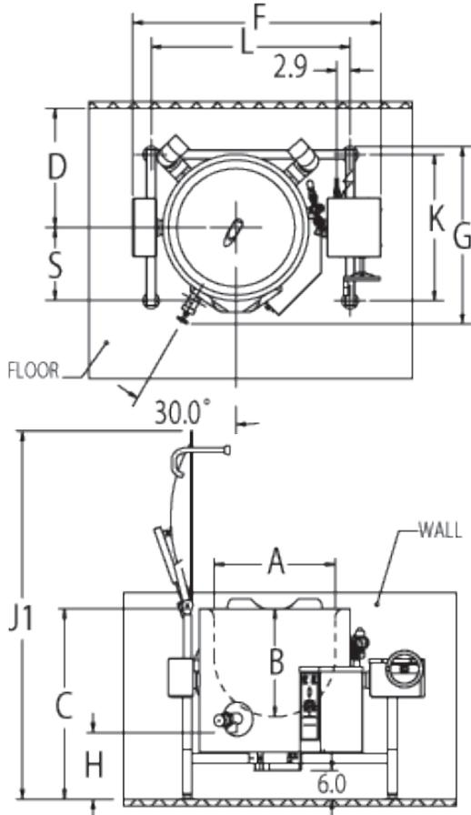
\*Dimensions on these drawings are applicable when using an optional 2" diameter draw-off valve. If a 3" diameter draw-off valve is required, contact AccuTemp for applicable dimensions.
