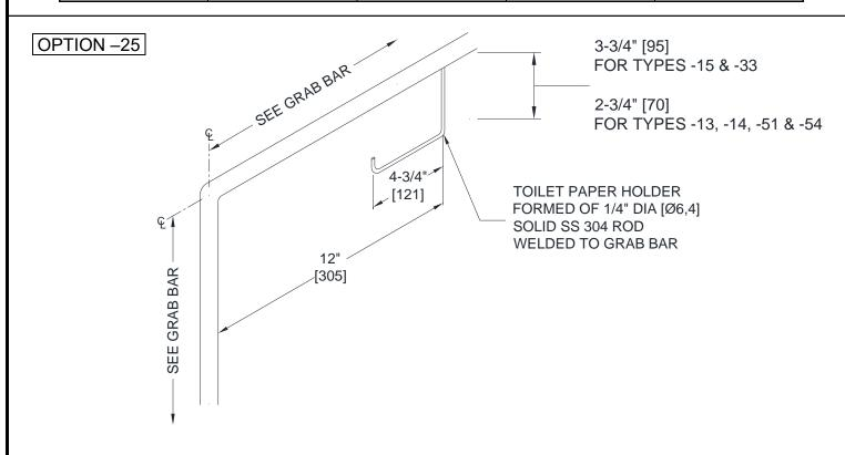
Option -25 Toilet Paper Holder is welded on to Grab Bars of the Swing Up or Swing Away configurations 3413, 3451, 3454 and Fixed Types -15, -33
