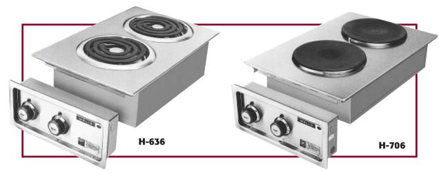
**Wells H-636 and H-706 Built-in hotplates** offer versatility with a choice of heating elements. The flat, spiral elements on the H-636 provide a wide cooking area for more surface contact and are self-cleaning. The solid cast-iron elements on the H-706 are engineered for uniform heat distribution, which is ideal for heating stock pots.
