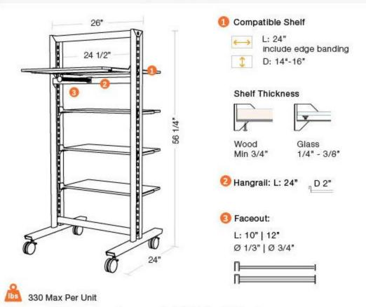
The max weight load is based on an evenly distributed weight load.
