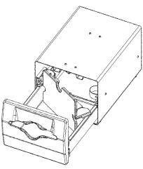
TO REMOVE DRAWER FOR CLEANING Push on left side of push plate while pulling on the right side. When the right side pops out, remove push plate.
