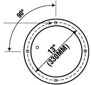
**NOTE: FOUR 1/2" O.D. MOUNTING HOLES SPACED ON 13" DIA. BY OTHERS**
