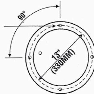
NOTE: FOUR 1/2" O.D. MOUNTING HOLES SPACED ON 13" DIA. BY OTHERS.
