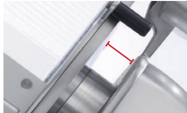
Increased gap between blade and machine body
