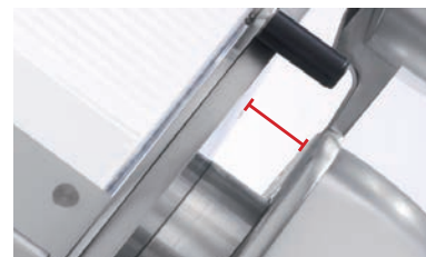
Increased gap between blade and machine body
