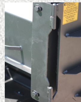
Adjustable Front hinge to insure proper Seal
