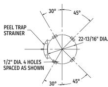
PLAN VIEW OF PEEL TRAP SHOWING HOLES IN LEGS FOR BOLTING TO FLOOR WHEN REQUIRED.
