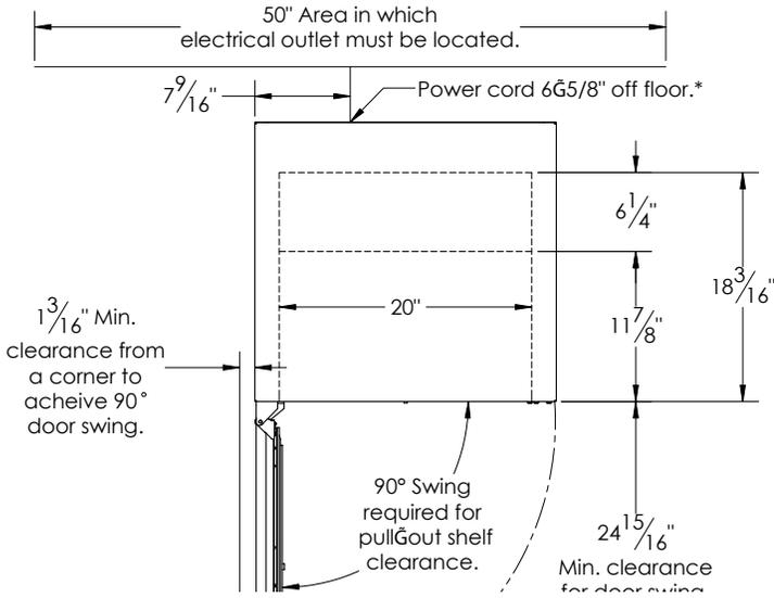
\* $\bar{G}$  Leg leveler can add 3/4" to these dimensions when fully extended.
