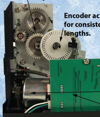
Inside View of Gears and Motor
