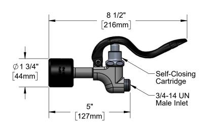
Flow Rate: 1.20 GPM (4.5 L/min) @ 60 psi Spray Force: 7.7 Ozf (218 Gramf) @ 60 psi
