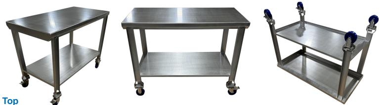
The top is formed of 11 gauge / 304 stainless steel and TIG welded complete to the frame. Our patented design eliminates all closed channels and requires no nuts, bolts, or threads for assembly.
