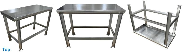
The top is formed of 11 gauge / 304 stainless steel and TIG welded complete to the frame. Our patented design eliminates all closed channels and requires no nuts, bolts, or threads for assembly.
